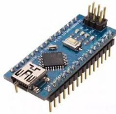
**Figura 3.8. Arduino Nano V3 (Xataca, 2017).**
