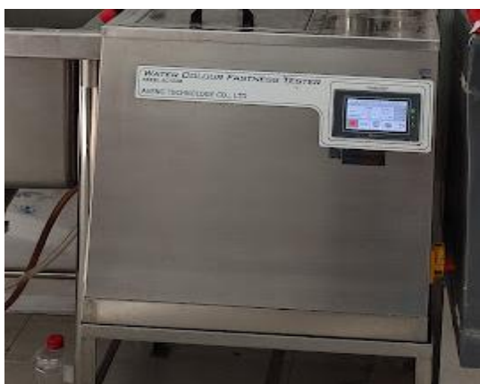
Lauderometro (WATER COLOUR FASTNESS TESTER) MODEL.AC10- 8A
